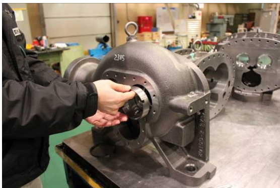
Photo 076 Attaching Balance Piston Sleeve
