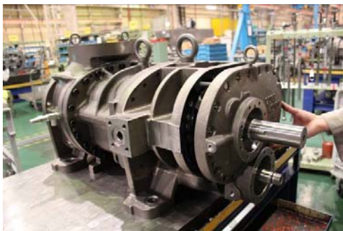
Photo 031 Removing Bearing Cover
