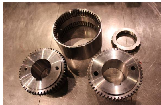
Photo 053 Current Parts of Gear Coupling
