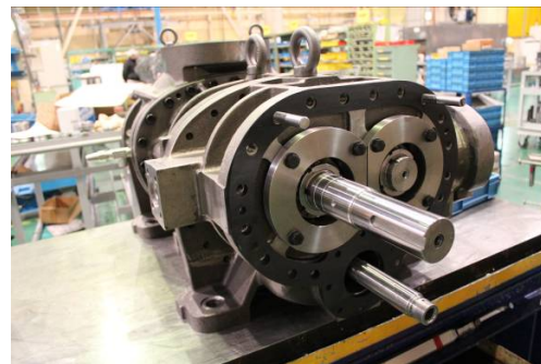
Photo 032 After the Bearing Cover is Removed
