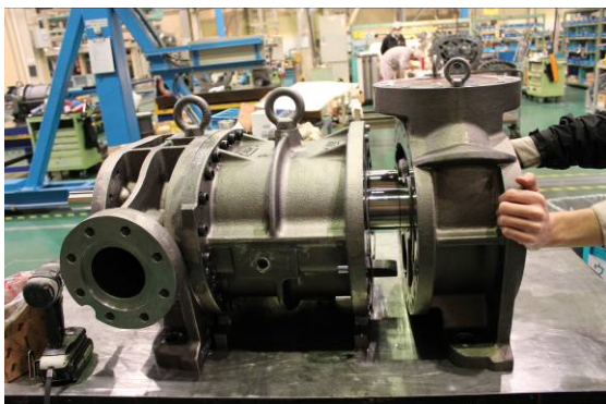
Photo 080 Assembling Low-stage Suction Cover
