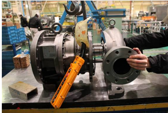
Photo 043 Pulling Out Suction Cover
