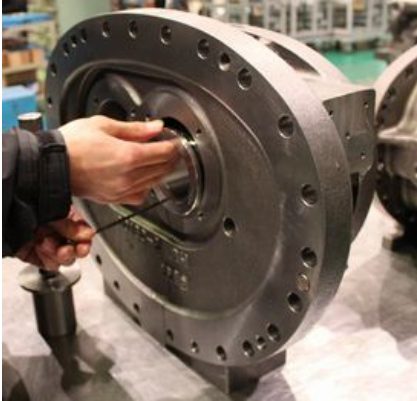
Photo 062 Attaching Main Bearing (High-stage)
