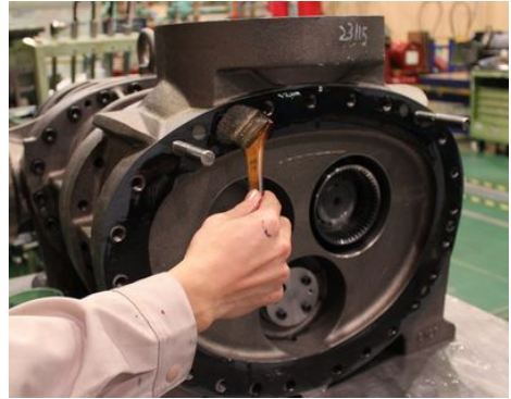
Photo 098 Attaching the Gasket onto the Low-Stage Flange Surface
