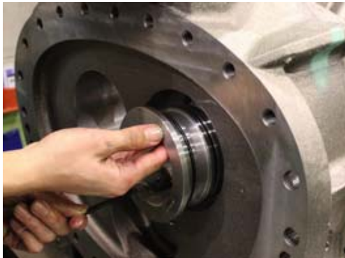
Photo 070 Attaching Side Bearing (Low-stage)
