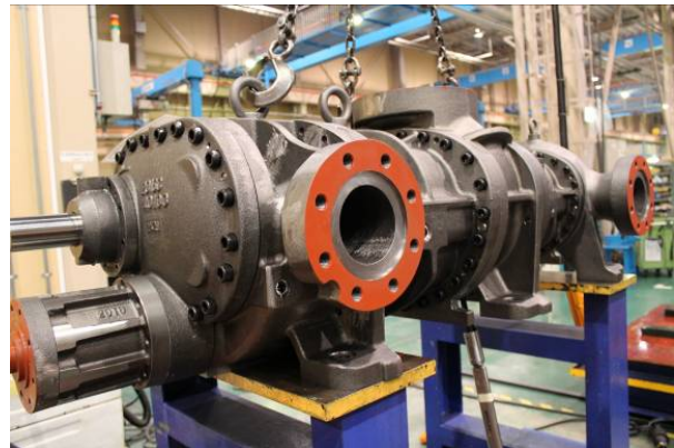
Photo 004 Lower-side Bolts for Fastening Rotor Casing
