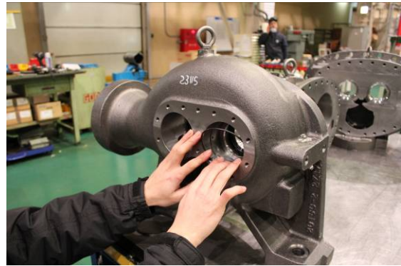
Photo 075 O-ring for Balance Piston Sleeve
