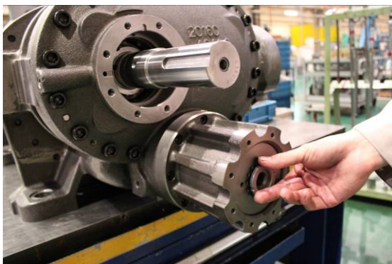
Photo 027 Removing Lock Nut
