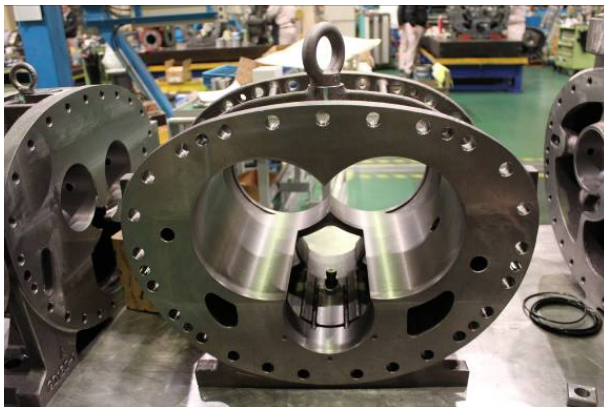
Photo 060 Guide Block Stem Inside the Casing
