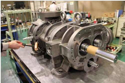
Photo 082 Driving In Alignment Pin for Positioning
