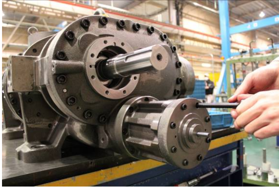
Photo 021 Loosening Bolts of Unloader Cylinder Cover
