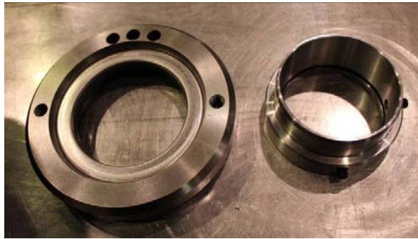
Photo 010 Oil Seal Retainer and Oil Seal Sleeve attached with O-ring
