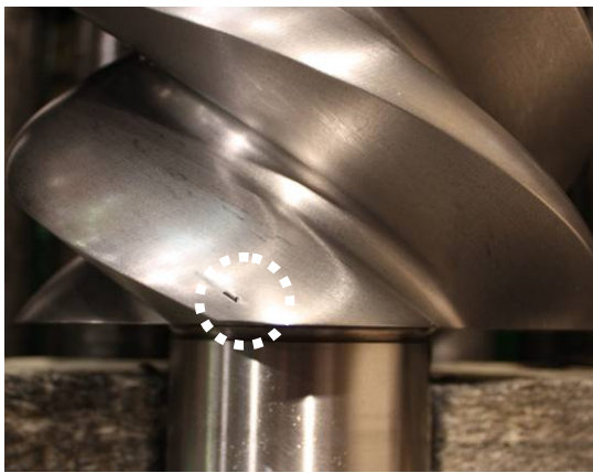
Photo 066 M Rotor Mating Mark
