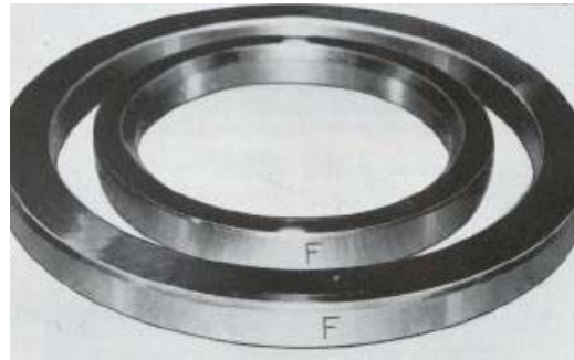
Photo 038 Stamp Marks on Spacer and Thrust Bearing Alignment Spacer
