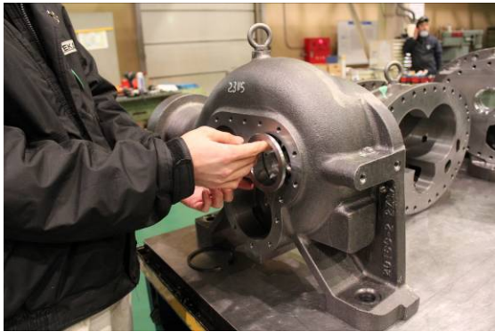
Photo 074 Attaching O-ring Spacer (High-stage)
