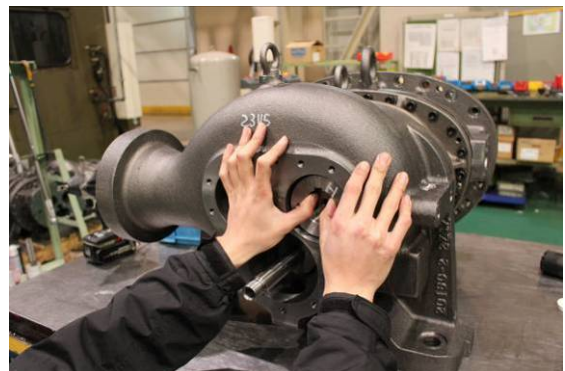
Photo 084 Attaching the Balance Piston
