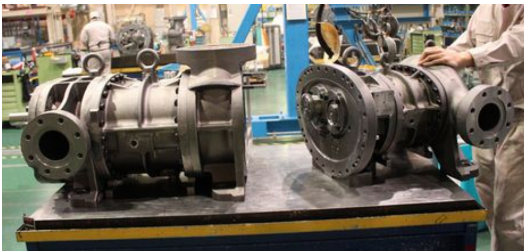
Photo 099 Attaching High-stage and Low-stage
