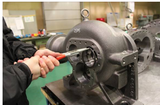
Photo 079 Attaching Stop Ring
