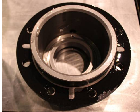
Photo 006 Seal Cover and Mating Ring
