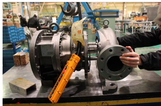
Photo 081 Assembling High-stage Suction Cover
