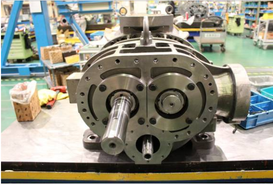
Photo 049 Low-stage Thrust Bearing Part
