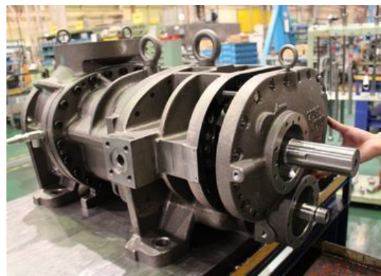
Photo 094 Attaching Bearing Cover
