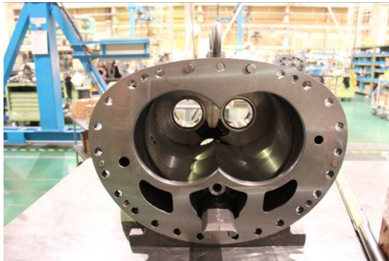
Photo 057 Low-stage Rotor Casing
